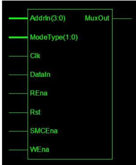
Fig.7: Block Diagram of Top Module
