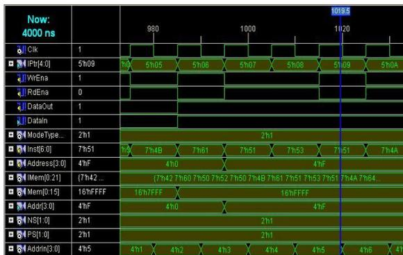
Fig.9: Simulation Waveform of Execution of 2<sup>nd</sup>-6<sup>th</sup> Instruction
