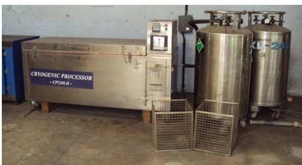
Figure 1: Cryogenic Processor
