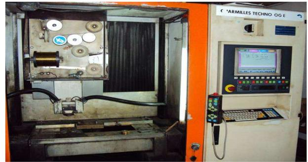
Figure 2: WED Machine Tool
