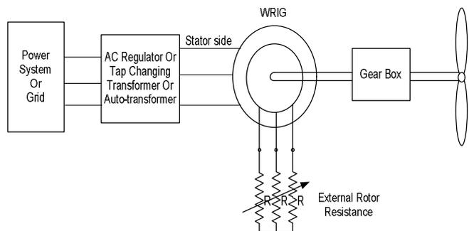
Fig. 4 Circuit topology of the combined input voltage and slip power control scheme
