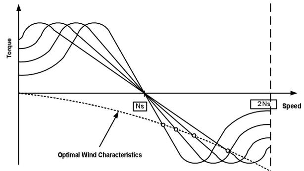
Fig. 3 Characteristics of a WRIG with rotor resistance control
