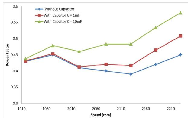
Fig.10 Power factor versus speed
