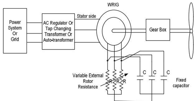
Fig. 6 Circuit topology of the proposed scheme
