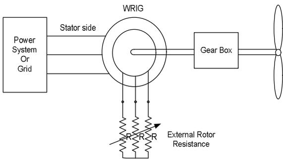
Fig. 2 Rotor resistance control of a wound rotor induction generator
