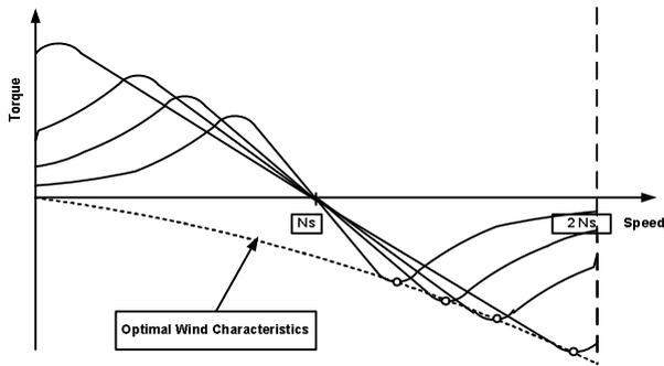
Fig. 5 Characteristics of a WRIG with rotor resistance as well as stator voltage control
