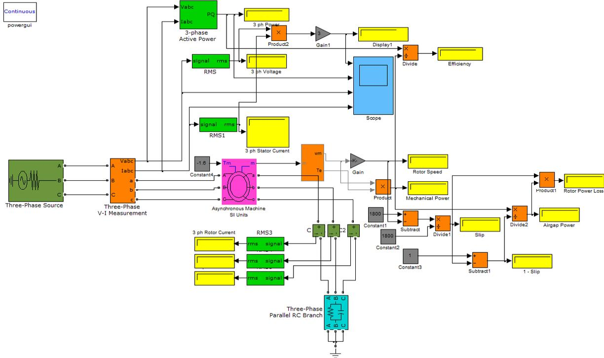
Fig.7 MATLAB Simulation model of WRIG feeding power to grid
