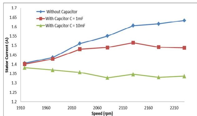
Fig.11 Stator current versus speed
