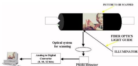
Fig1.1: The schematic diagram of image scanner-digitizer diagram
