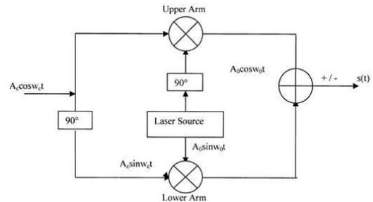
Fig .2 Illustration of OSSB modulation using phase shift method
