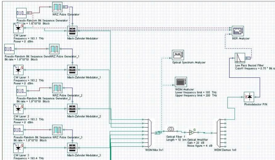
Fig .3 Simulation Setup of WDM
