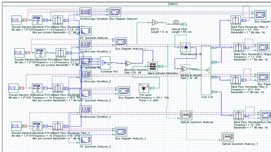
Fig .4 Simulation Setup of SCM
