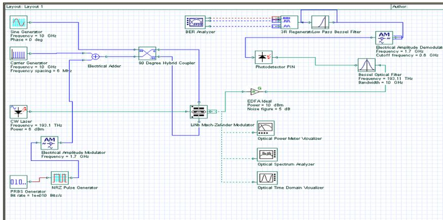
Fig .5 Simulation setup of SCM employing OSSB modulation
