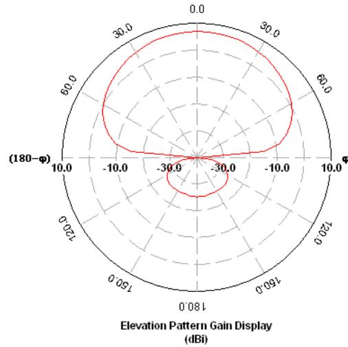
Figure 4: Radiation pattern for  $L_s=4.025\text{mm}$
