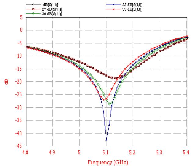
Figure7: Return loss of the proposed antenna.
