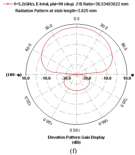
Figure 3: Radiation pattern for  $L_s=3.825\text{mm}$
