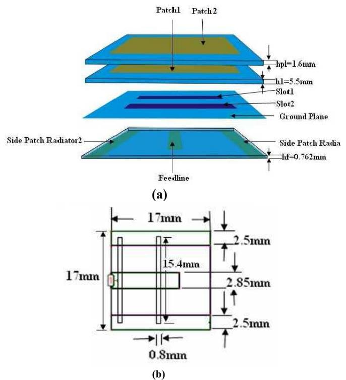
Figure1: Double slot coupled microstrip antenna
