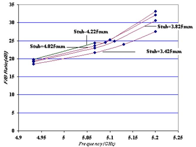
Figure 6: Plot between F/B ratios at different stub lengths versus frequency
