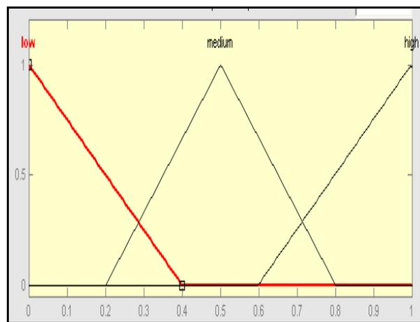
Figure 1. Input Variable 'Signal power'
