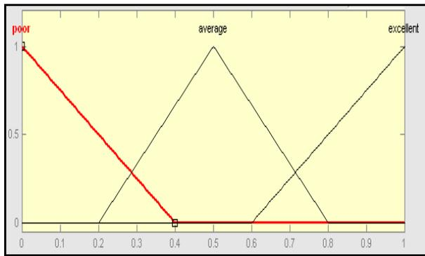
Figure 2. Input Variable 'Delay'
