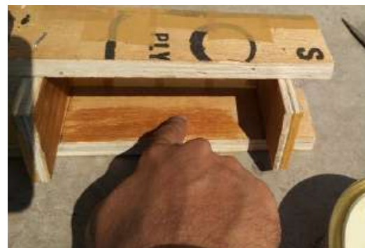
Fig.10 coating plywood mould with release agent (wax)
