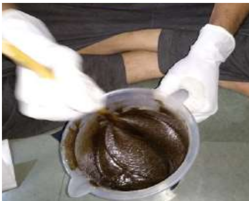
Fig.7 mixing and stirring process of composite
