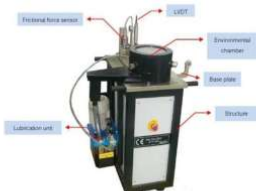
Fig.14 ducom pin-on-disc tribometer
