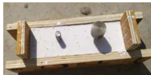
Fig.11 mixture of silicon is poured in plywood mould
