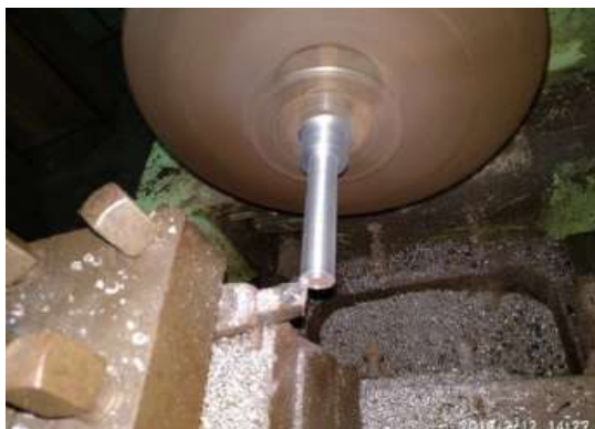
Fig.8 preparing prototype of 12mm diameter on lathe
