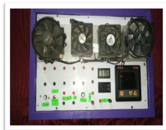
Fig:3 Arrangement of six TEGs with cold side and hot side in a board
