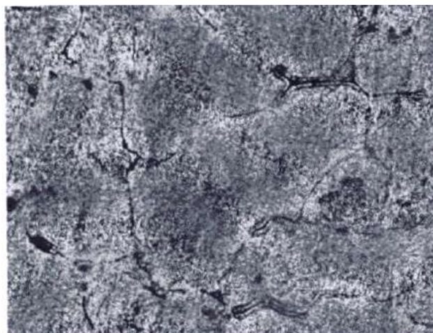
Figure-5 Microstructure of sample containing 8% Cu
