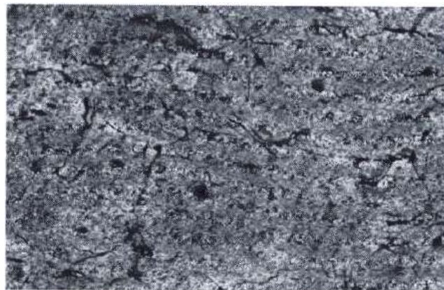
Figure-5 Microstructure of sample containing 8% Cu
