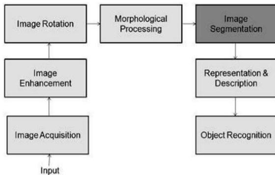
**Figure 1:** Fundamental Steps in Digital Image Processing
