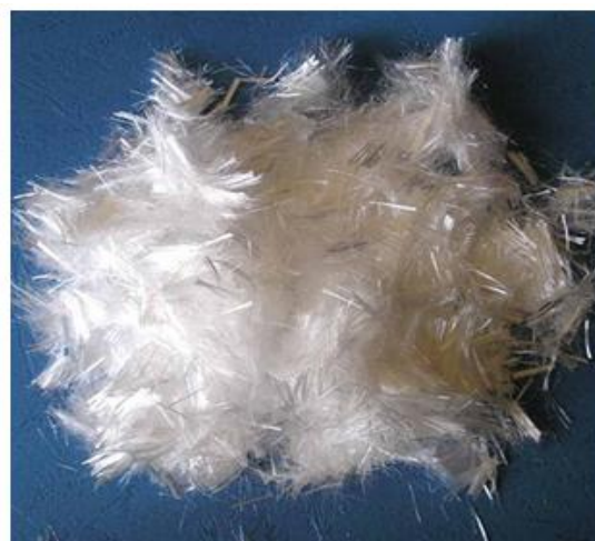
Polypropylene Fibre (Recron 3s)Property Values Cut length 6mm or 12mm
