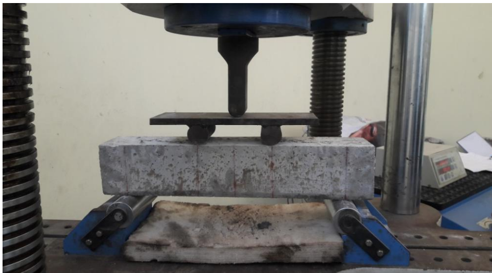
Fig.4 UNIVERSAL TESTING MACHINE WITH BEAM SPECIMEN
