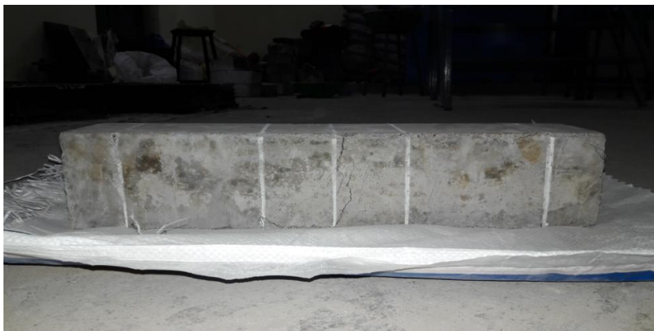
Fig.4 FAILURE AFTER FLEXURAL TEST
