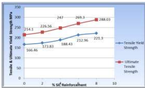
Fig-5: Plot of Tensile Yield Strength and Ultimate Tensile Strength with % SiC
