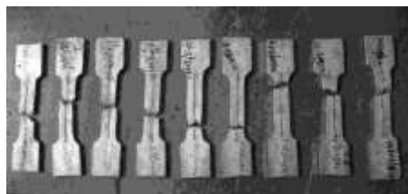
Figure 2: Tested tensile Al/SiC composite specimens
