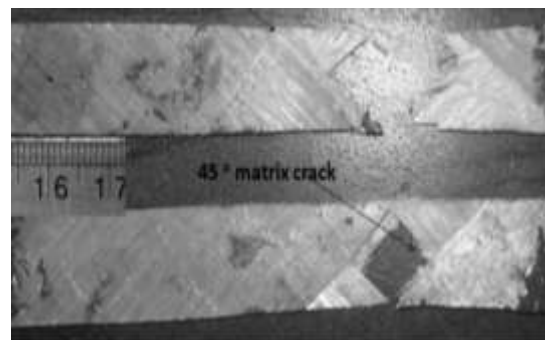
Fig. 6. Failure mode of [45/-45] 2s Shear test
