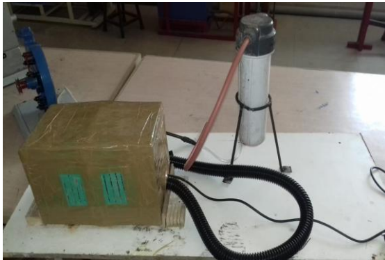
Fig. 6: Model of Oil Mist Lubrication system.
