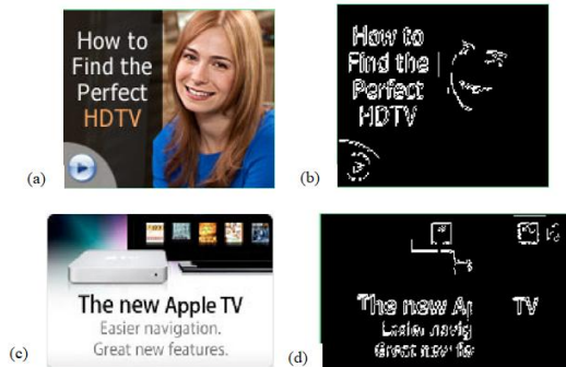
Figure 8. Extraction process of Connected Component Algorithm, (a) and (c) are original images, (b) and (d) respective output
