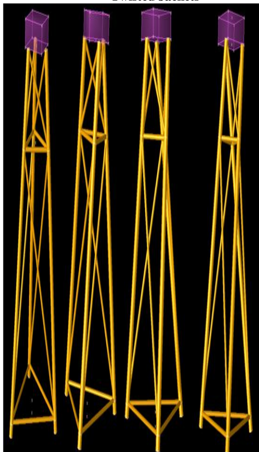
Fig. 3: Modified Twisted Jacket models in SACS with 0°, 30°, 60° & 90° twisting angles
