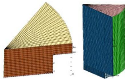
Fig.2.3 Sector mesh of in-cylinder fluid domain at TDC
