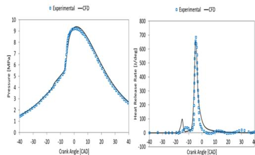
Fig.3.1 comparison of cylinder pressure and Heat release rate CFD and experimental values
