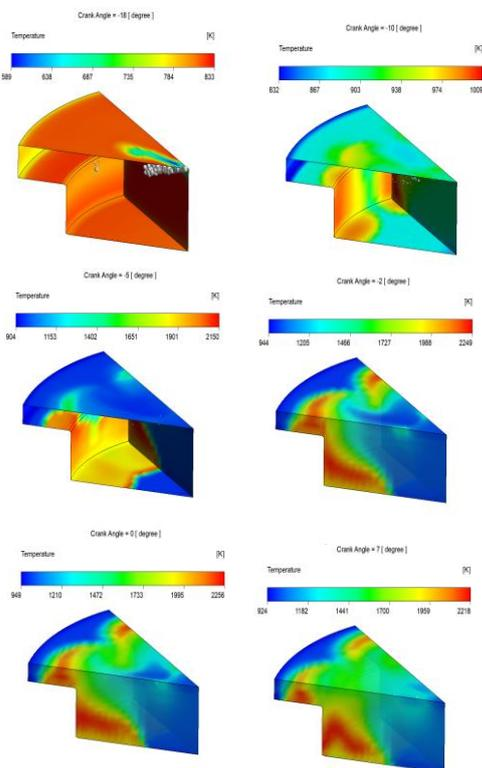
**Fig.3.2** Fuel particles and in cylinder temperature contours of flat piston bowl
