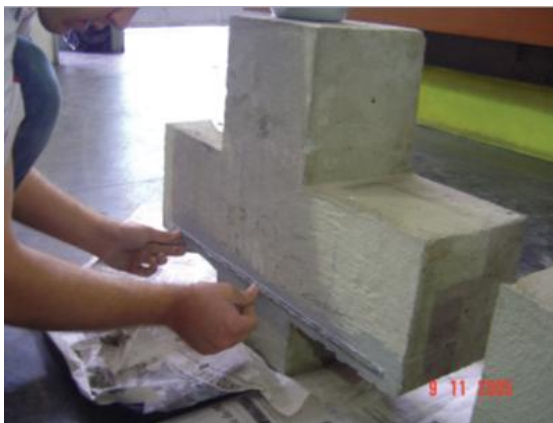
b) strengthening of corbels Figure 3. Near-surface mounting fiber-reinforced polymer (a) of beams and (b) short corbels.
