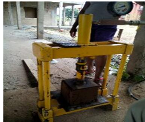
Plate B2: Enerpac Compressive Testing Machine
