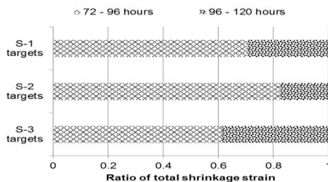
**Fig. 5** Ratios of shrinkage strains monitored between 72 to 96 hours and 96 to 120 hours for S-1 to S-3 targets in C-0.55 mixture specimen
