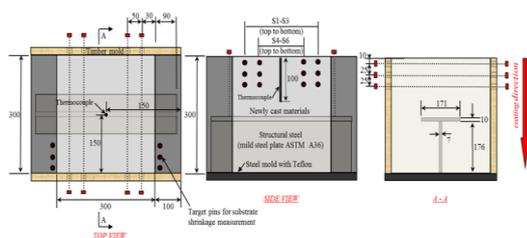
Fig. 1 Composite Type C specimens comprising structural steel, hardened concrete substrates and freshly cast cementitious mixtures
