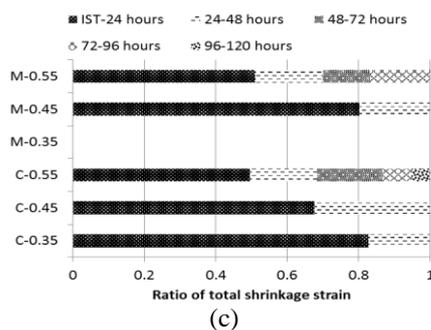
**Fig. 4** Ratios of S-1 (a), S-2 (b) and S-3 (c) shrinkage strains developed in Type C specimens between consecutive 24-hour intervals up to 120 hours of monitoring for OPC mixtures under “sealed” condition
