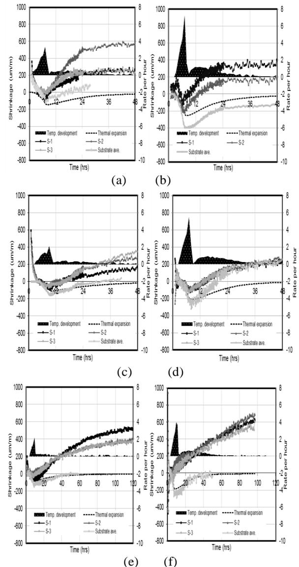
**Fig. 2** Shrinkage strains of Type C specimens cast using concrete and mortar mixtures with w/c ratios of (a, b): 0.35, (c, d): 0.45 and (e, f): 0.55 under “sealed” condition
