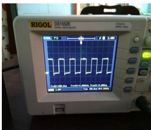
Fig 7 Duty cycle (gate pulses) to the Switch in buck converter
