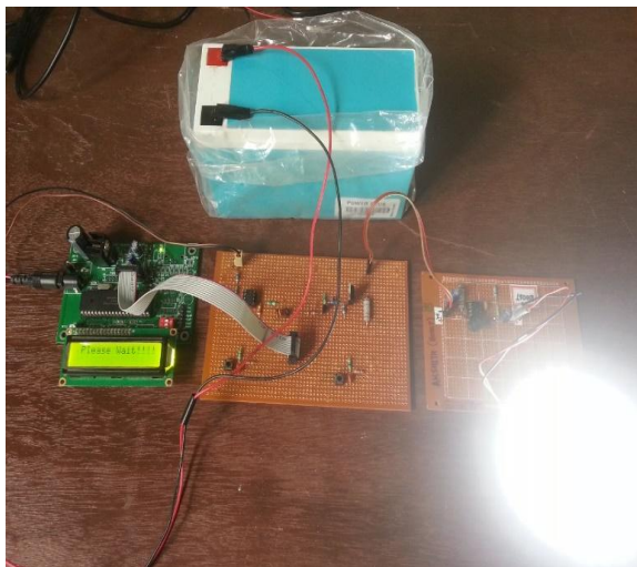
Figure-1.7: Experimental Setup With The Boost Converter And LED Load
