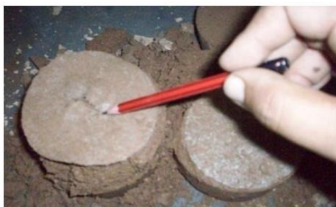
Plate.3. Rupture Failure Of Fabric Reinforcement
