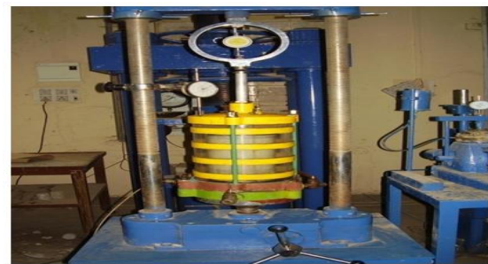
Plate 2. Large Triaxial Test–Experimental Set Up
