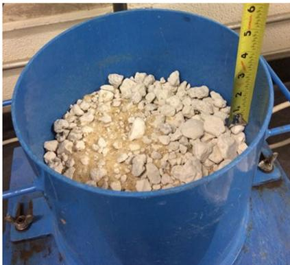
Fig. 8 Second Step of The Vibrated Packing Test on Ternary Aggregate Blends, Measuring the Distance Between the Top Vibrated Sample and Rim.
