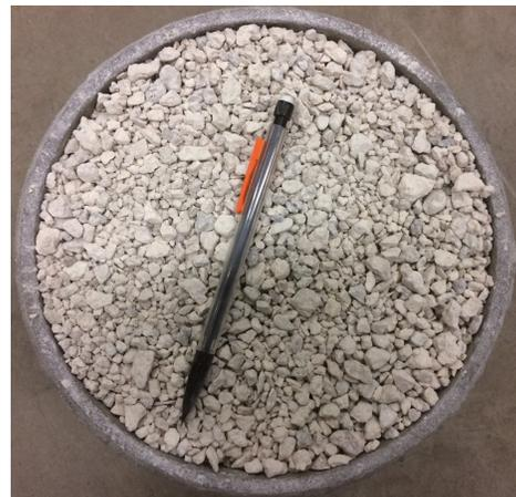
**Fig. 6** Traditional Dry-Rodded Packing Test.
