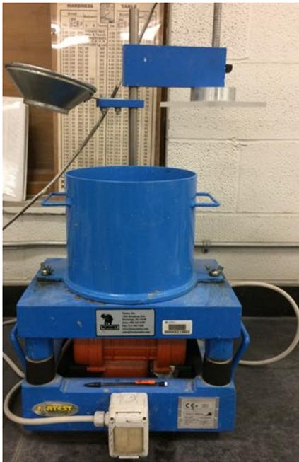
Fig. 7 Vebe Apparatus for Vibrated Aggregate Packing Test.
