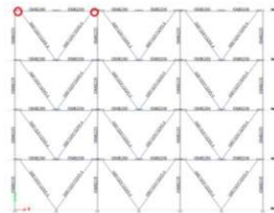
Figure3:Sectionofsteelbuilding showing VshapedbracingandEDBincorners.
