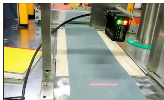
Fig. 5.2 Experimental set up for Automatic Weight based rubber cutting machine
