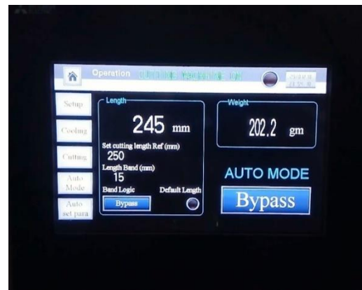
Fig 7.8 HMI Display of Auto Mode
