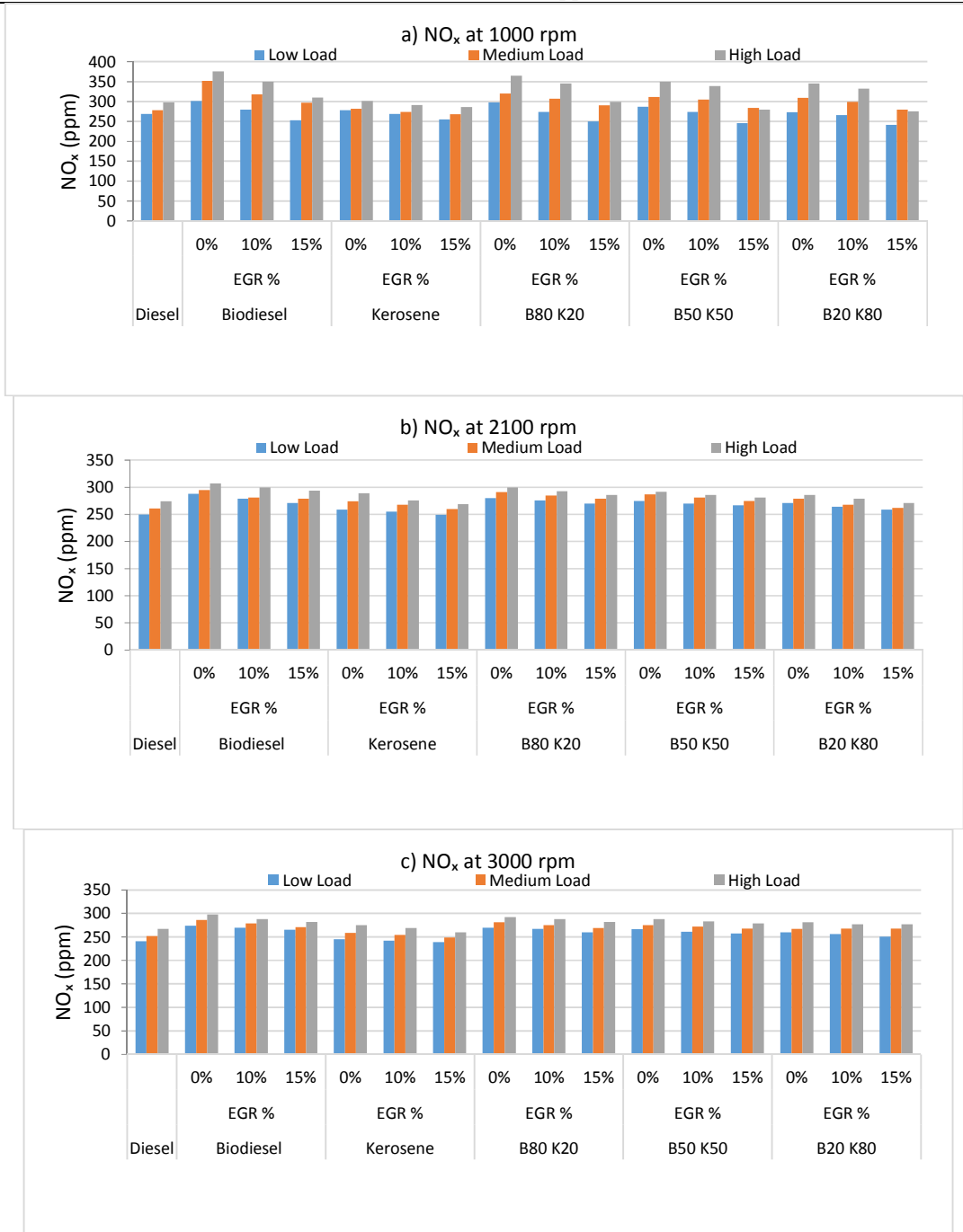
Fig. 4: NO x emission of different fuel blends with and without EGR at a)1000 rpm, b)2100 rpm, and c) 3000 rpm
