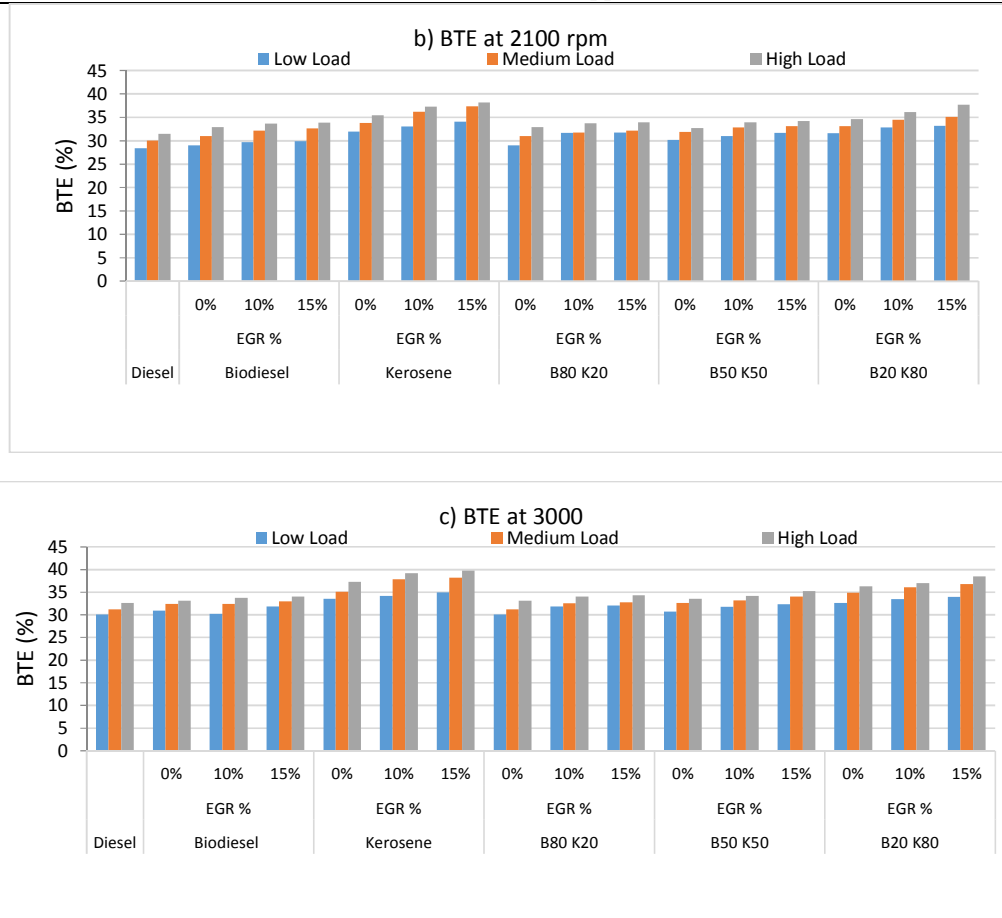
Fig. 3: BTE of different fuel blends with and without EGR at a) 1000 rpm, b) 2100 rpm, and c) 3000 rpm
