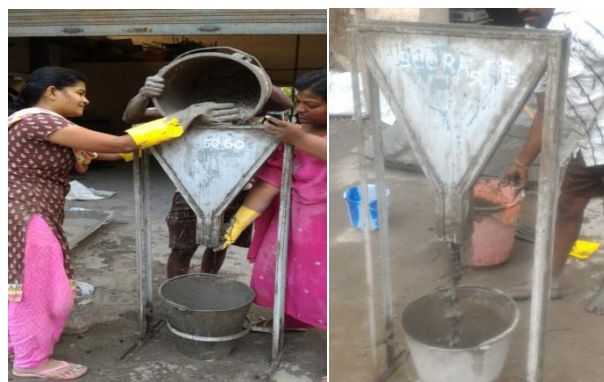
Fig 3: Apparatus set up and flow diagram for V funnel flow test
