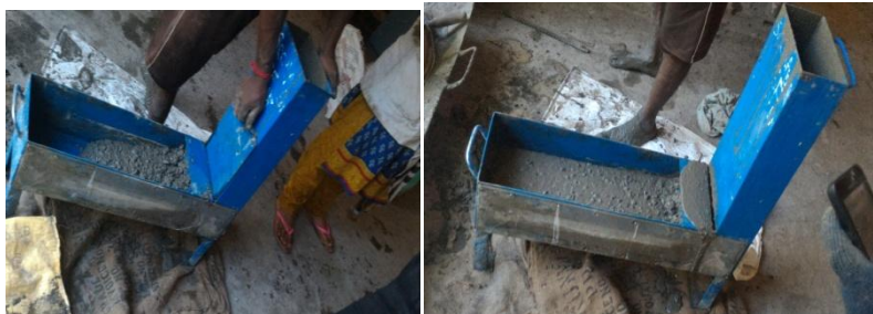
Fig 4: Apparatus set up and flow diagram for L box test
