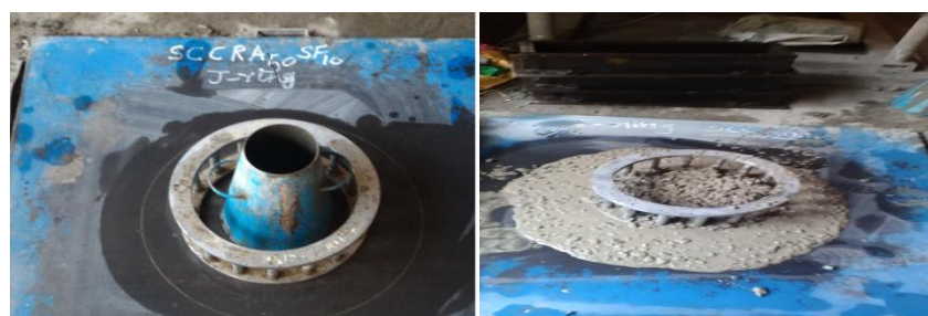
Fig 2: Apparatus set up and flow diagram for J ring flow test
