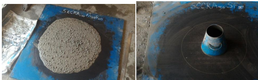
Fig 1: Apparatus set up and flow diagram for slump flow test
