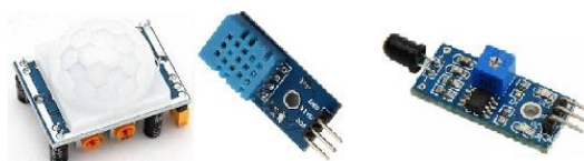
Figure 3. HCSR501, DHT11 and UVFlame (760nm-1100nm) Sensors
