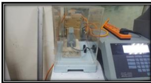
Fig. 6. Thermal Conductivity Test.
