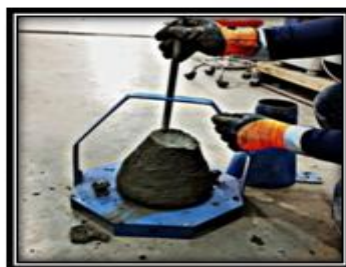
Fig. 5 Slump Test of reference Concrete mix
