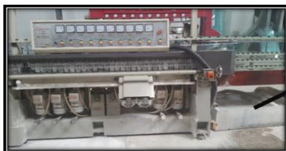
Fig. 3. Grinding and polishing edges on flat glass machine
