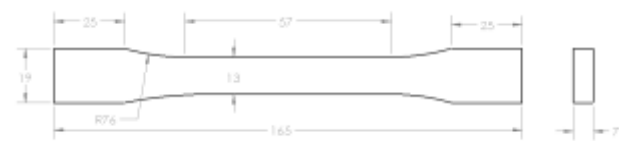
Fig: 4 Tensile Test Specimen (ASTM D – 638)
