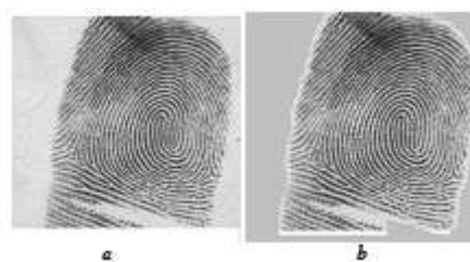
Fig. 2. Fingerprint image before (a) and after (b) segmentation
