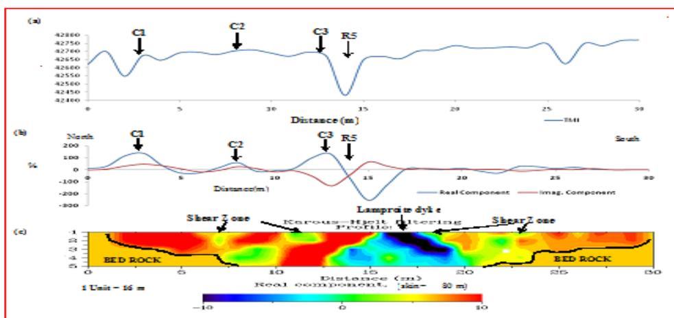
**Figure:11** (a) Total Magnetic Intensity, (b) Fraser filter Real and Imaginary Components (VLF) and (c) Karous Hjelt current density pseudo section along the profile Ramadugu (R5 - 16°49'50.2", 79°17'17.8")
