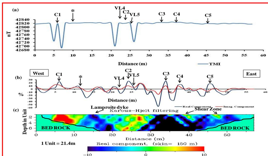
**Figure: 18** (a) Total Magnetic Intensity, (b) Fraser filter Real and Imaginary Components (VLF) and (c) Karous Hjelt current density pseudo section along the profile Vattikodu (VL4-16°54'58.2",79°05'24.2",VL5 - 16°54'58.2", 79°05'24.3" \* Probable Lamproites)
