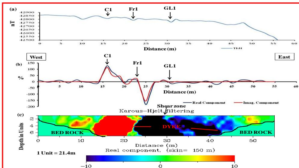
**Figure:15** (a) Total Magnetic Intensity, (b) Fraser filter Real and Imaginary Components (VLF) and (c) Karous Hjelt current density pseudo section along the profile Gundrapally (GL1 - 16°56'35.9", 79°02'38.6")
