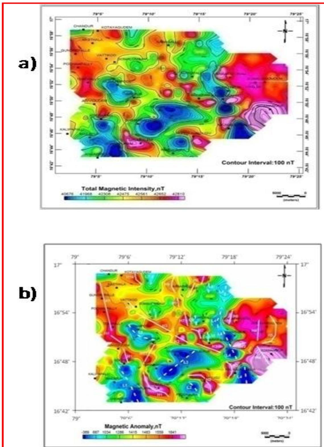
Figure 3:- (a) Total magnetic Intensity of the study area, (b) IGRF of corrected magnetic anomaly of the study area.
