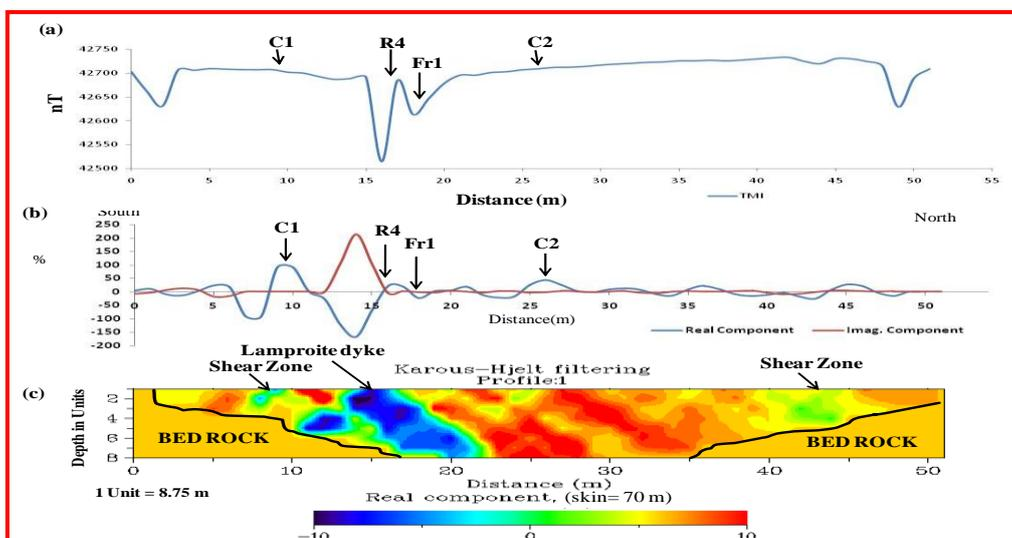
**Figure: 10** (a) Total Magnetic Intensity, (b) Fraser filter Real and Imaginary Components (VLF) and (c) Karous Hjelt current density pseudo section along the profile Ramadugu (R4 - 16°50'18.7", 79°16'37.7")
