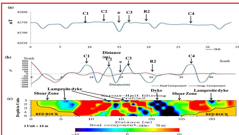
**Figure: 8** (a) Total Magnetic Intensity, (b) Fraser filter Real and Imaginary Components (VLF) and (c) Karous Hjelt current density pseudo section along the profile Ramadugu (R2 - 16°50'13.3", 79°16'38.0", \* Probable Lamproites)
