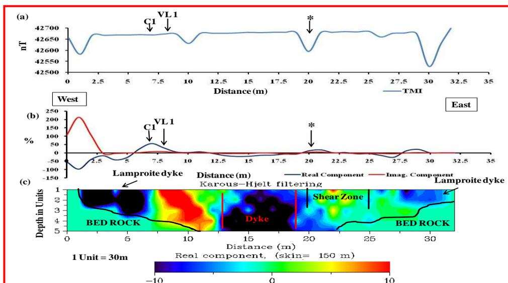
**Figure16** (a) Total Magnetic Intensity, (b) Fraser filter Real and Imaginary Components (VLF) and (c) Karous Hjelt current density pseudo section along the profile Vattikodu (VL1-  $16^{\circ}55'03.5''$ ,  $79^{\circ}05'01.2''$ , \* Probable Lamproites)
