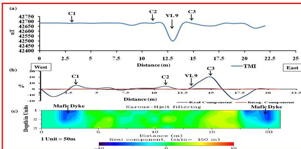
**Figure: 20** (a) Total Magnetic Intensity, (b) Fraser filter Real and Imaginary Components (VLF) and (c) Karous Hjelt current density pseudo section along the profile Vattikodu (VL9- 16°55'02.5", 79°05'13.00")
