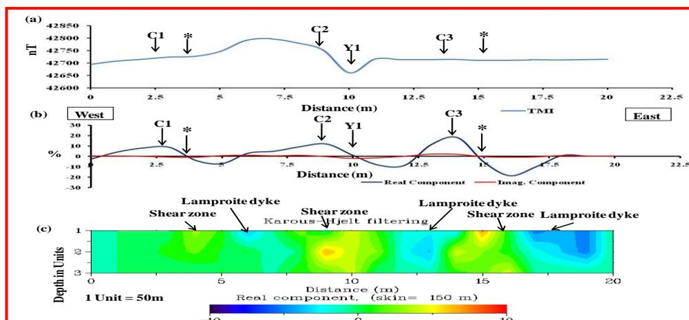
**Figure:12**(a) Total Magnetic Intensity, (b) Fraser filter Real and Imaginary Components (VLF) and (c) Karous Hjelt current density pseudo section along the profile Yacharam (Y1 - 16°51'12.9", 79°15'32.1", \* Probable Lamproites)
