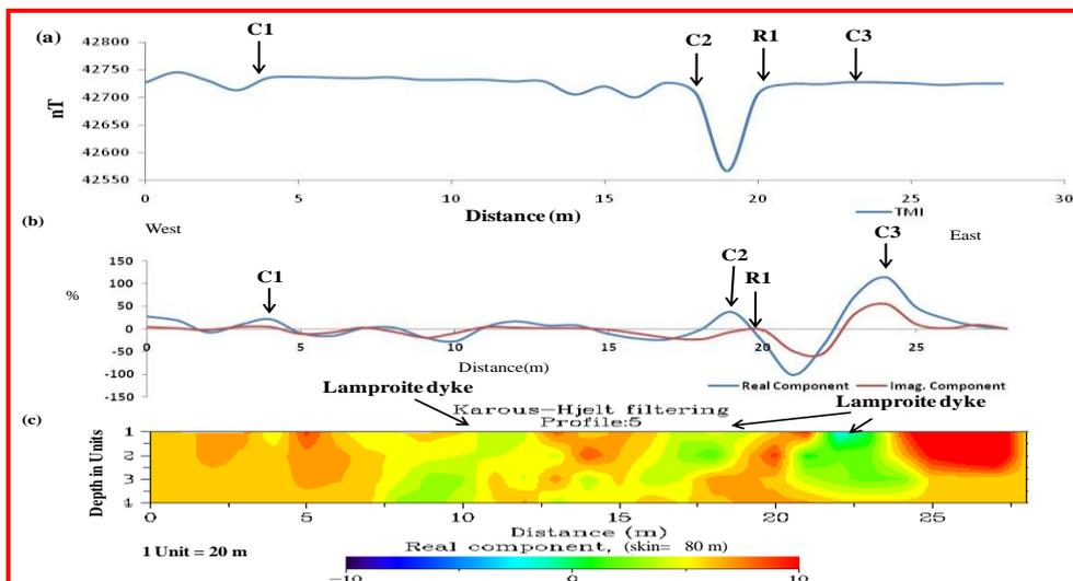
**Figure: 7**(a) Total Magnetic Intensity, (b) Fraser filter Real and Imaginary Components (VLF) and (c) Karous Hjelt current density pseudo section along the profile Ramadugu (R1 - 16°50'17.1", 79°16'40.9")
