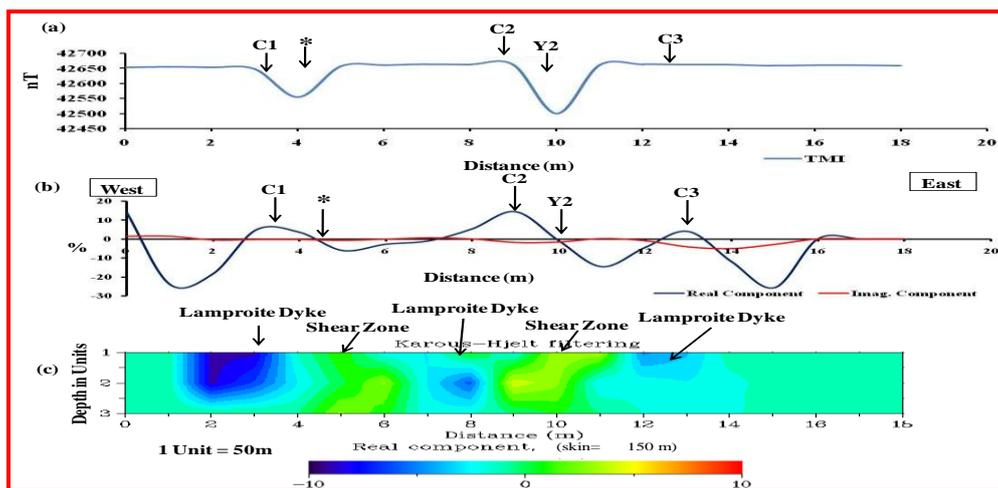
**Figure:13** (a) Total Magnetic Intensity, (b) Fraser filter Real and Imaginary Components (VLF) and (c) Karous Hjelt current density pseudo section along the profile Yacharam (Y2 – 16°51'09.9", 79°15'15.2", \* Probable Lamproites)
