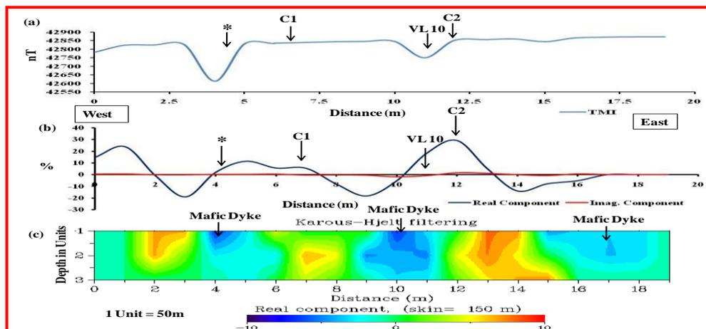
**Figure: 21** (a) Total Magnetic Intensity, (b) Fraser filter Real and Imaginary Components (VLF) and (c) Karous Hjelt current density pseudo section along the profile Vattikodu (VL10 -  $16^{\circ}55'00.8''$ ,  $79^{\circ}05'15.5''$ , \* Probable Lamproites)
