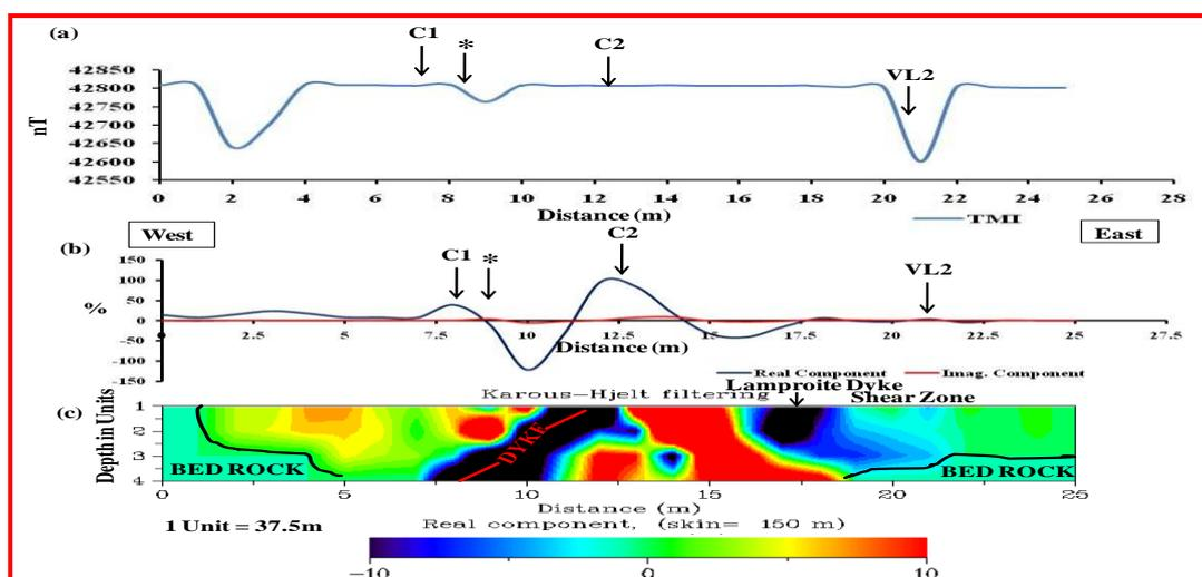
**Figure: 17** (a) Total Magnetic Intensity, (b) Fraser filter Real and Imaginary Components (VLF) and (c) Karous Hjelt current density pseudo section along the profile Vattikodu (VL2 -  $16^{\circ}54'55.4''$ ,  $79^{\circ}05'23.3''$ , \* Probable Lamproites)
