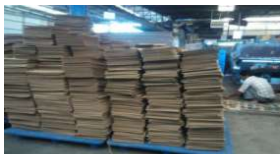
Fig. 6 Corrugated sheets are placed over pallets
