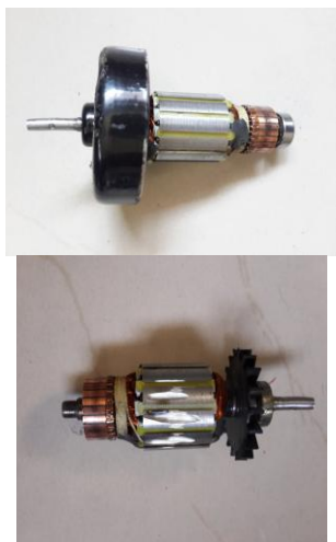
Fig 6. Images of Healthy Rotor & Damaged Rotor bars
