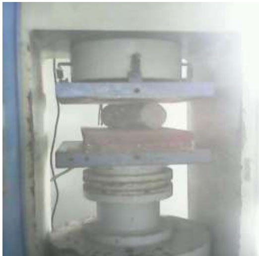
Figure 6.3 split tensile testing machine
