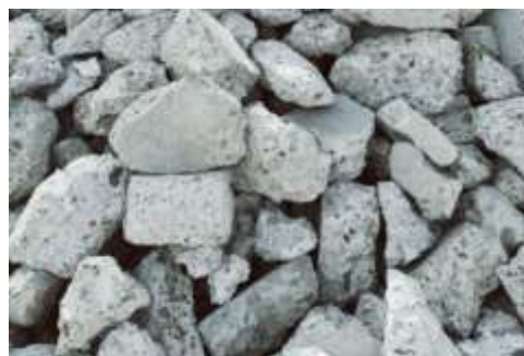
Figure 2.2 demolished concrete waste.
