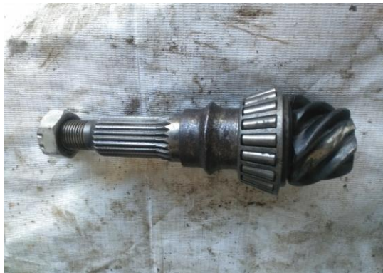
Fig.3 Test pinion with one broken teeth
