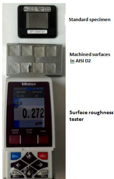
Figure3: Surface roughness testing AISI D2 sample
