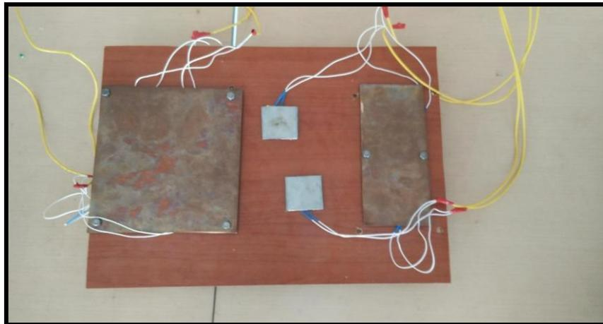
Fig. 3: Experimental setup after attaching Copper heat spreaders
