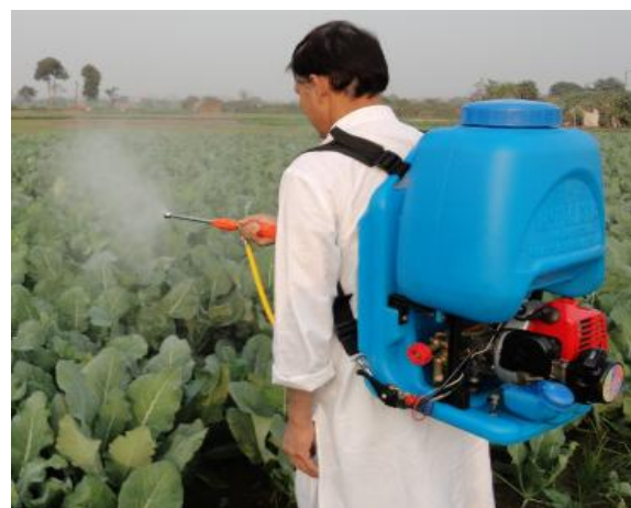
Fig.3: Engine operated sprayer
