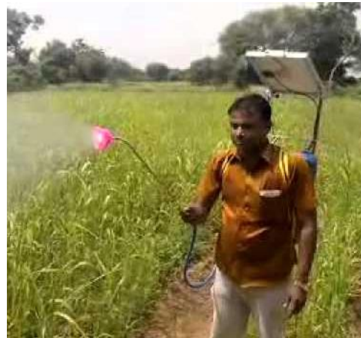
Fig 5: Manual Solar Powered Sprayer
