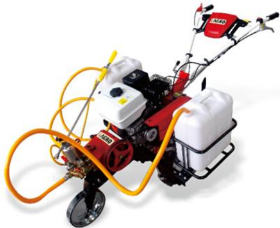
Fig. 4: Power Tiller sprayer
