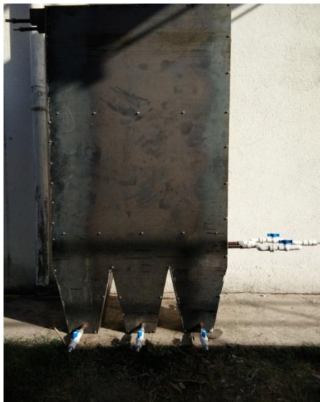
Fig. 2 Setup of Tube settler Module
