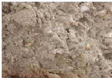
Fig.8 Structure of Papercrete
