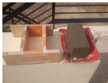
Fig.4 Papercrete mould and brick
