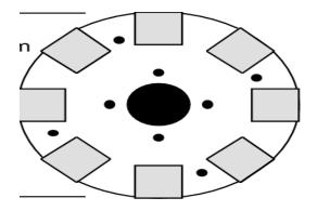
Each magnet rotor is built on a wooden or hard plastic disk, 12cm thick. Do not use aluminum or stainless steel for this disk! The disks have to be made of magnetic material. The disk has holes to mount it to them. At the center of the disk is a 2mm diameter hole. The magnet plates must be flat, not warped. It is not easy to cut the outer circle without warping the plate. The magnets will be placed on the round disk [6].
