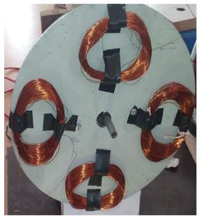
The total assembly of the stator which has shown above diagram. After completion of fixing copper coils on stator, remove the insulation on copper coil, then make a connection of all coils either as a series or parallel but you should take care about connection the coils should be same direction i.e. all coils should be clockwise, not one coil clockwise and another is counterclockwise.
