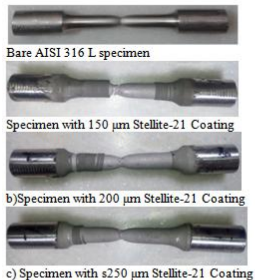
Fig 5: Different Specimens after Tensile Test
