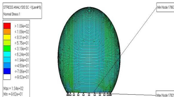
Fig 4 Normal Stresses  $\sigma_1$  on the bottom panel
