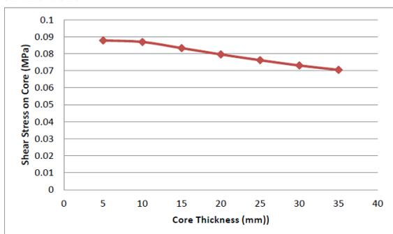
Fig 7 Shear stress on core for varying core thickness
