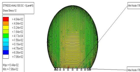
Fig 5 Shear Stresses on the core panel
