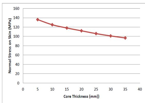
Fig 6 Normal stress on skin for varying core thickness
