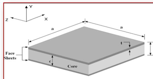
Fig 1 A typical sandwich panel construction
