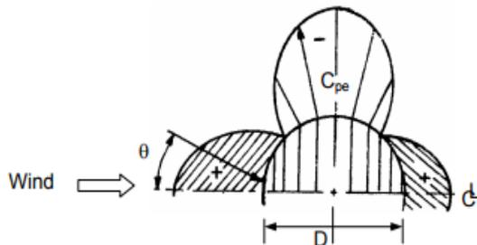
**Fig2** External Pressure Distribution coefficients around spherical structures
