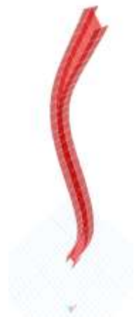
Figure 12: Mode shape 10 for shear wall
