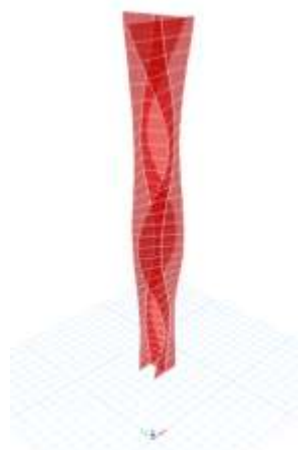
Figure 10: Mode shape 8 for shear wall
