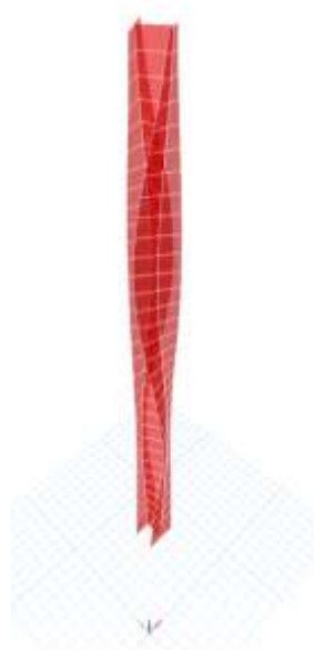
Figure 9: Mode shape 7 for shear wall
