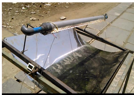
Fig.6.Experimental setup with thermocouple materials and S.S parabolic trough reflector
